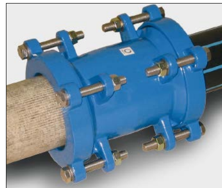
Fig. 10.4: Wide-tolerance coupling for transitions between materials (fibre-cement pipe on the left, PE pipe on the right) where bolts are fastened to the body
